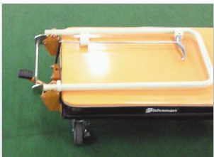
The BX15 handle is collapsible.
